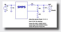
The .step command is useful for sweeping a variable across a range of values in a single simulation run. The variable can be temperature, a model parameter, a global parameter or in our case an independent source. These steps can be defined as linear, logarithmic or as a list of specific values.
