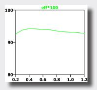
Of course, calculating efficiency is only one example. The .meas and .step commands can be combined in countless other ways to characterize your analog circuit designs.
